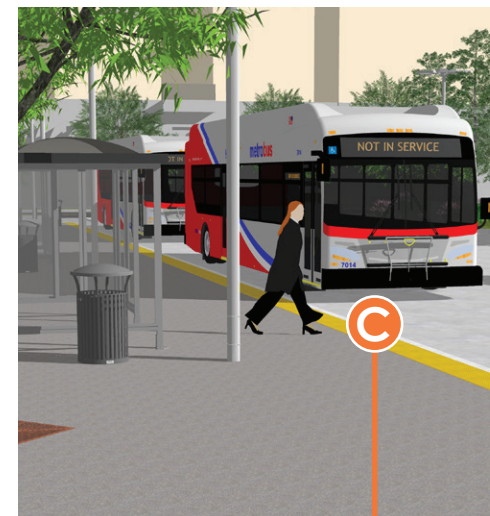
Bus boarding lanes that are at least 12' wide and 50' long for each standard bus (70' for articulated buses)
