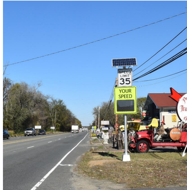
Radar-activated speed limit sign on Route 301 in the Town of Port Royal.
