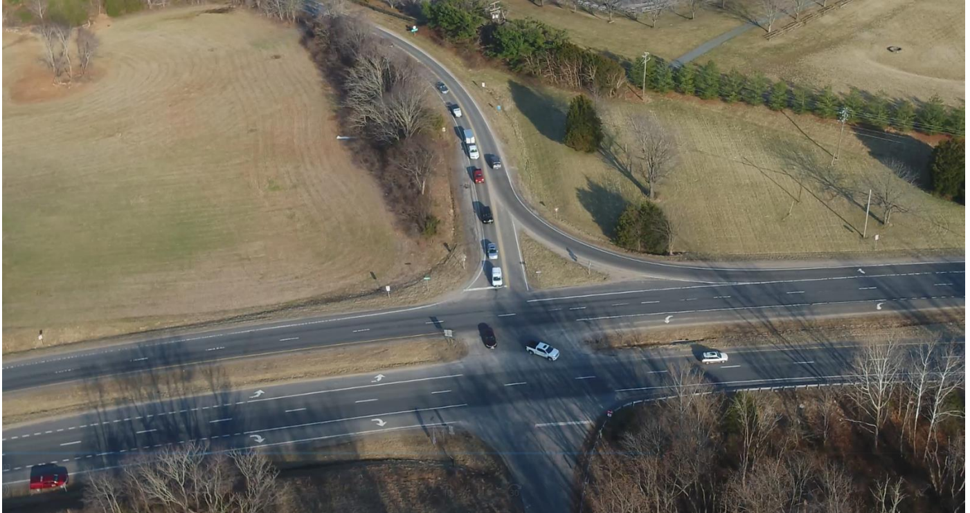
Figure 15: Aerial View of Route 245 Westbound Left Turn PM Peak Hour Queue onto Southbound US 17
