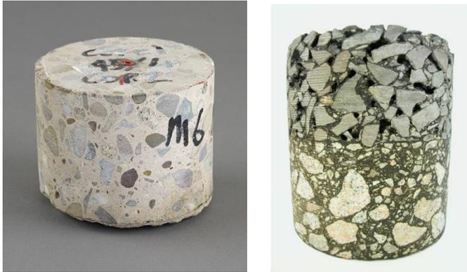
Sample concrete & asphalt core samples
