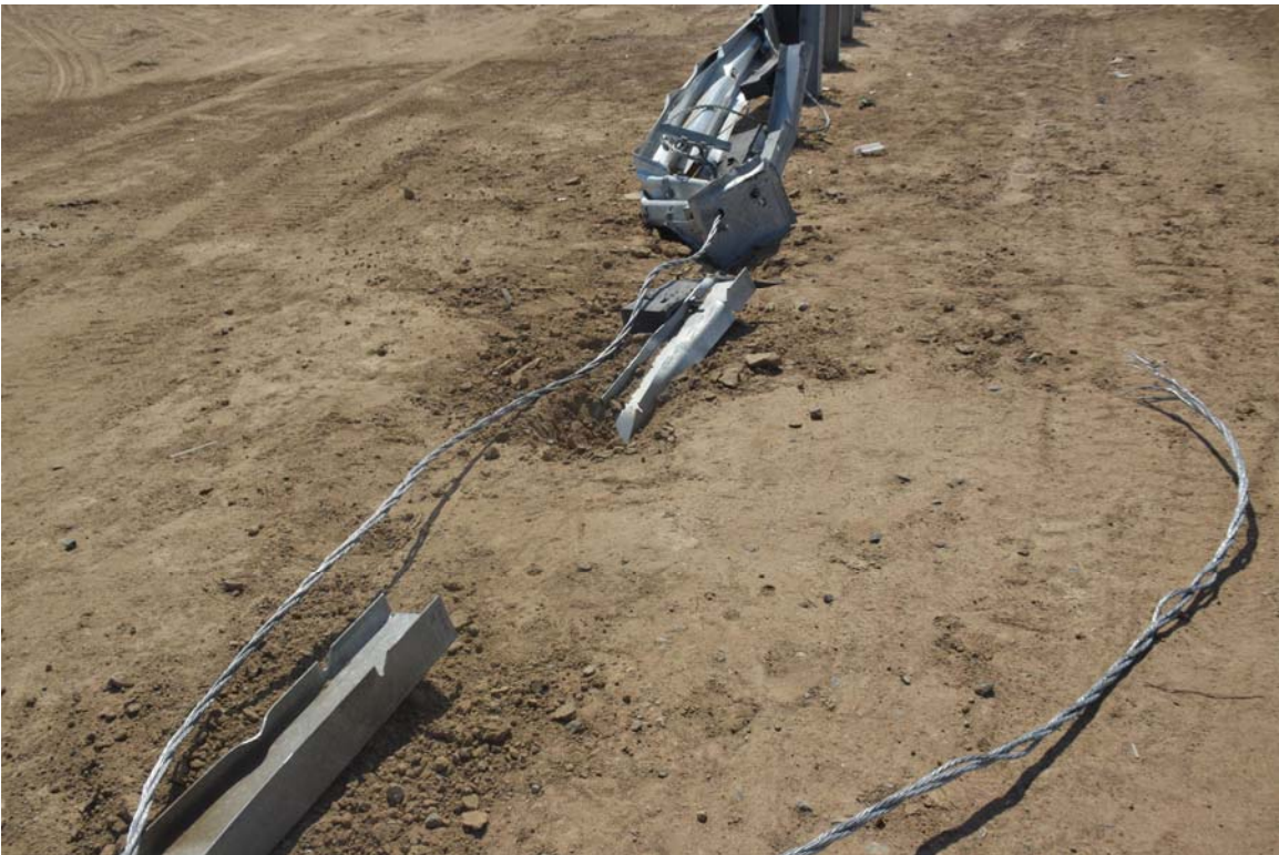
FIGURE 36. Test Article Damage
