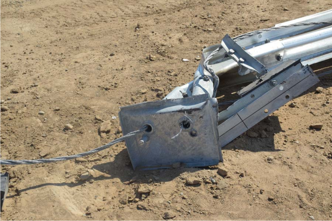
FIGURE 35. Test Article Damage
