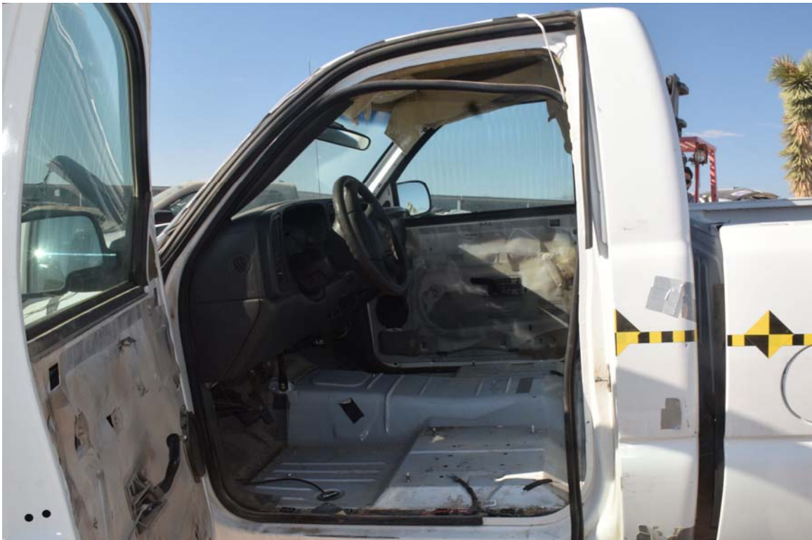
FIGURE 54. Post-Test Driver Side Occupant Compartment
