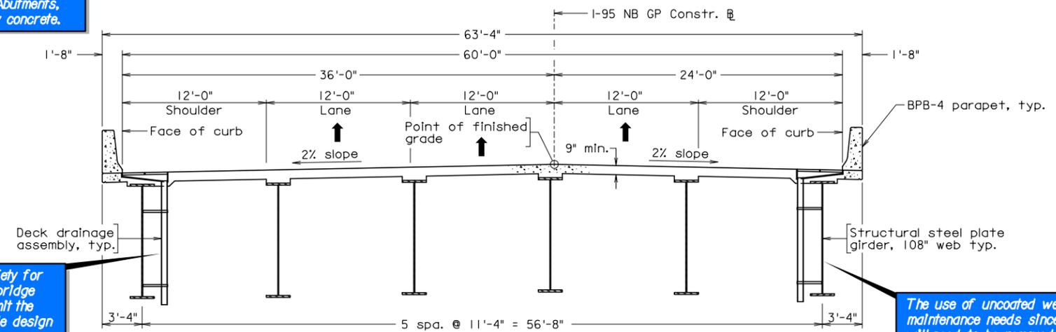
In order to provide reasonable safety for the passage of vehicular traffic, bridge deck drains will be provided to limit the maximum spread for the applicable design storm to the shoulder area with no encroachment into the travel lanes.
