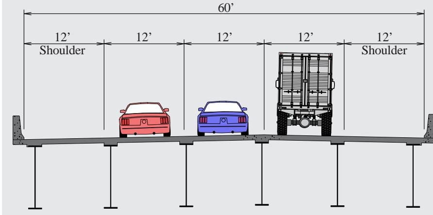
The proposed structure will have a clear roadway width of 60', accommodating three 12' lanes, a 12' outside shoulder, and a 12' inside shoulder. A VDOT Standard 42" Concrete F-Shape Parapet (BPB-4) will be used along both sides of the bridge, which has an Adjusted Test Level of TL-5 and meets all RFP requirements.
