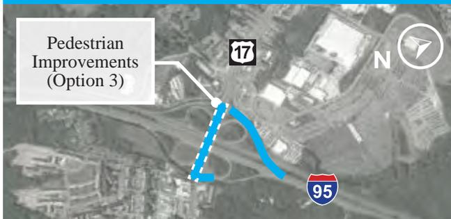
NB Route 17 will require a minor shift to the inside to allow for the widening and tie in to occur. In this phase, work can also begin along Route 17 Ramp B. Lanes here will be required to be reduced to 14' to allow for the proposed construction to occur.
