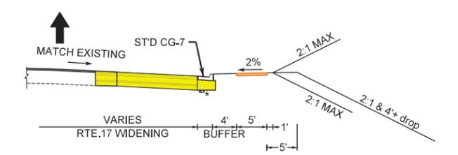
CURB AND GUTTER SECTION WITH SIDEWALK
