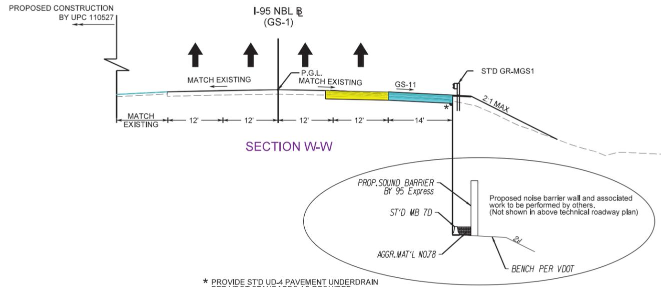
\* PROVIDE STD UD-4 PAVEMENT UNDERDRAIN PER VDOT STANDARDS AS REQUIRED.
