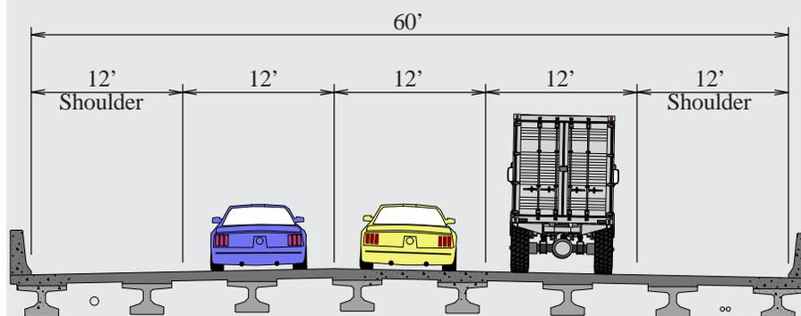
The proposed structure will have a clear roadway width of 60', accommodating three 12' lanes, a 12' outside shoulder and a 12' inside shoulder. A VDOT standard 42" Concrete F-Shape Parapet (BPB-4) will be used along both sides of the bridge, which has an Adjusted Test Level of TL-5 and meets all RFP requirements.
