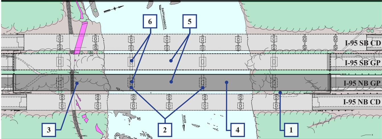
1. The horizontal clearance between the existing I-95 NB bridge and the new I-95 NB GP Lanes bridge meets the minimum horizontal clearance requirements specified in the RFP, which will provide VDOT sufficient horizontal clearance to inspect the underside of the new bridge carrying the I-95 NB GP Lanes over the Rappahannock River bridge using an under bridge inspection unit staged along the right shoulder of the I-95 NB GP lanes.
