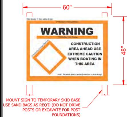
MOUNT SIGN TO TEMPORARY SKID BASE USE SAND BAGS AS REQ'D (DO NOT DRIVE POSTS OR EXCAVATE FOR POST FOUNDATIONS)
